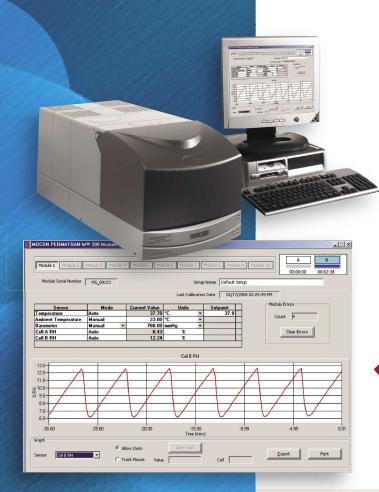
The new, easy to use, PERMATRAN-W Model 398 is the latest water vapor transmission rate system in a long line of quality systems available from MOCON, the world leader in permeation technology. This simple, low maintenance system conforms to the new ASTM Standard E-398 and produces the accurate and reliable data the industry has come to expect only from MOCON.
