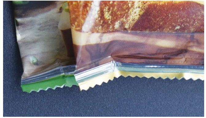
Rejected package with folds in the seal.
